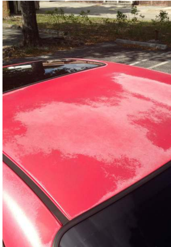
Paint damage caused by unprotected exposure to pollution and sun
